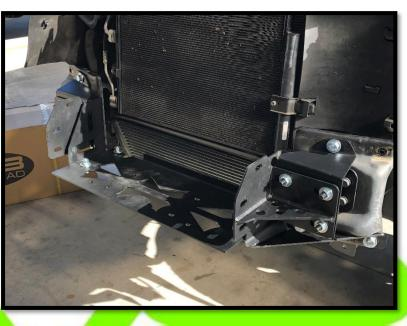
4. Begin by mounting the bracket/winch plate onto the frame of the truck. Most bumpers will utilize factory installation hardware for this. Then mount the center section to winch plate. Be sure to leave all hardware loose. Note: If installing winch, install it now.
