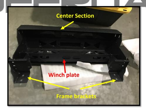
5. Once center section is on, attach wings using supplied hardware. If the studs for the wings are welded on to the center section, use flat washers, split lock washers, and the correct nuts. If not, use the short thick bolts M10/M12 along with the same washers to attach wings. Leave loose until final steps. Note: If your wings allow lights, install them prior to placing on wings.
