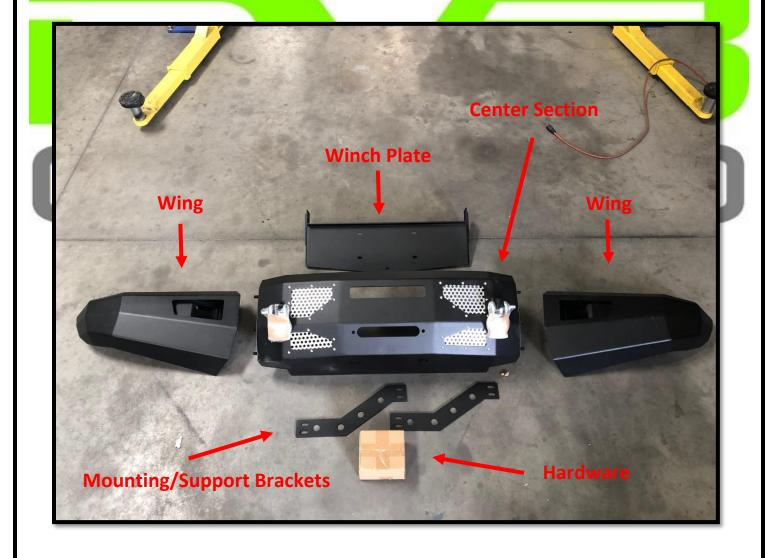
3. If your bumper has a detached winch plate, this will mount to the frame of the vehicle prior to mounting the center section. Examples below.
