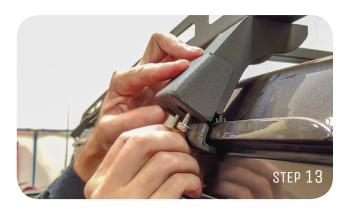
STEP 14: Making sure the rack is centered on the top, tighten up the front and back gutter clamps on each side first. This ensures the 4 other clamps move as needed to fit properly. Then tighten the 4 middle clamps.
