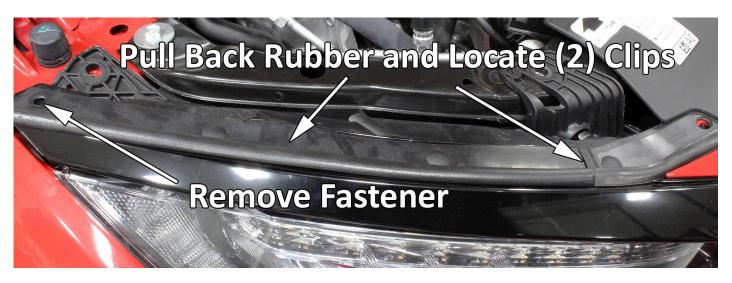
2. On each headlight remove (1) fastener as shown and locate (2) clips under rubber trim. Pull forward on plastic trim and push down on clips to free trim from head light.
