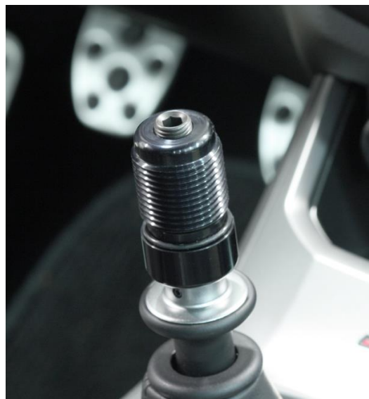
This picture shows outer knob removed from adapter and set screw exposed and ready for adjustment.
