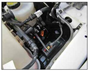
8. Connect the wiring harness to the boost module and connect the throttle pedal harness to the pigtail from the boost module.
