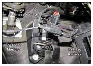
5. Connect the provided pedal harness into the factory harness and to the pedal assembly.
