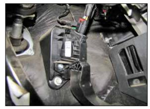
4. Locate the throttle pedal connector under the instrument panel. Release the red locking tab and disconnect the connector from the pedal assembly.
