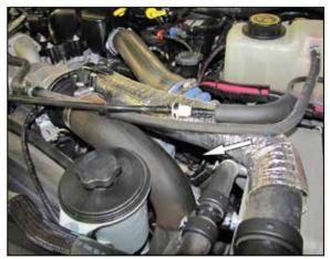
2. Locate the Fuel rail pressure sensor under the intercooler tube on the driver's side of the engine. Release the red locking tab and disconnect the factory wiring harness from the sensor. **NOTE: The throttle pedal pigtail is a 3-pin connector.**
