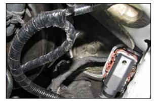
6. Create a small hole in the fire wall grommet and route the pedal harness through the hole into the engine compartment.
