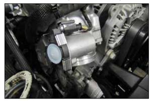
9. Reinstall the throttle body with the factory gasket and hardware. Reconnect the throttle body electrical connection.
