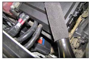
13. Secure the boost wiring harness to the boost module. Find a suitable location to secure the boost module and secure with the provided tie wraps.
