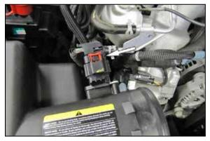
11. Reinstall the air filter housing so that the mounting studs insert into the mounting grommets. Reconnect the mass air sensor electrical connection.
