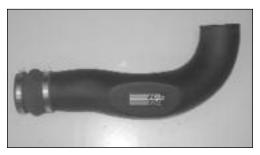
11. Install the silicone hump hose (08176) and hose clamps onto the K&N intake tube as
