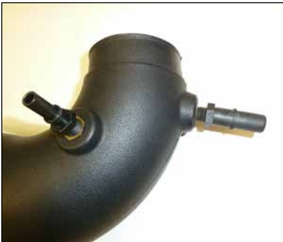
14. Install the provided quick disconnect fittings into the K&N intake tube as shown. Note: Some vehicles may only have one vent line, on those vehicles install the provided 1/4npt [lug in place of the smaller quick connect fitting.
