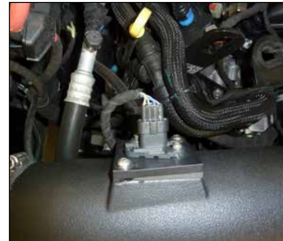
19. Reconnect the mass air sensor electrical connection.
