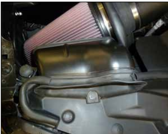
21. Reinstall the fresh air intake duct and secure with the factory push pin.
