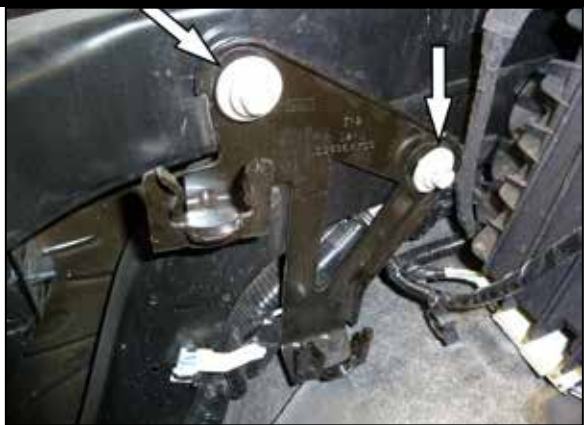
7. Remove the two bolts securing the air filter housing mounting brackets and then remove the bracket.
