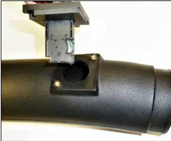
13. Install the mass air assembly into the K&N intake tube and secure with the provided hardware. NOTE: Be sure to install the sensor in the correct direction for proper operation.
