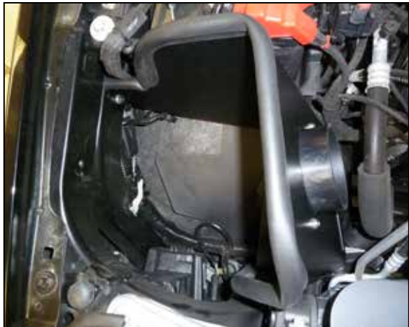
11. Install the heat shield assembly into the vehicle so the mounting post inserts into the factory mounting grommet and then secure with the provided hardware.
