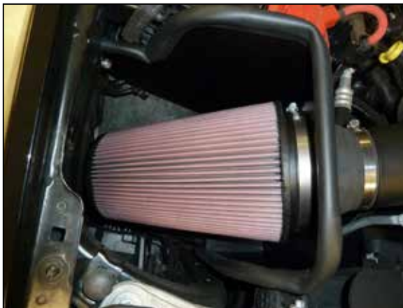
20. Install the K&N air filter and secure with the provided hose clamp.
