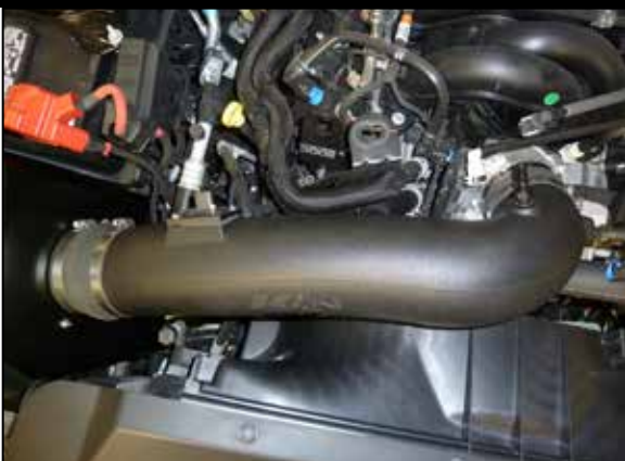
17. Install the K&N intake tube into the hump coupler and then connect to the throttle body, secure with the provided hose clamps
