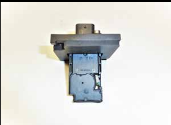
12. Install the provided gasket onto the mass air sensor adapter and then install the mass air sensor into the adapter and secure with the provided hardware.
