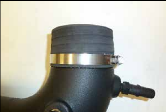
15. Install the provided straight coupler onto the K&N intake tube and secure with the provided hose clamp.
