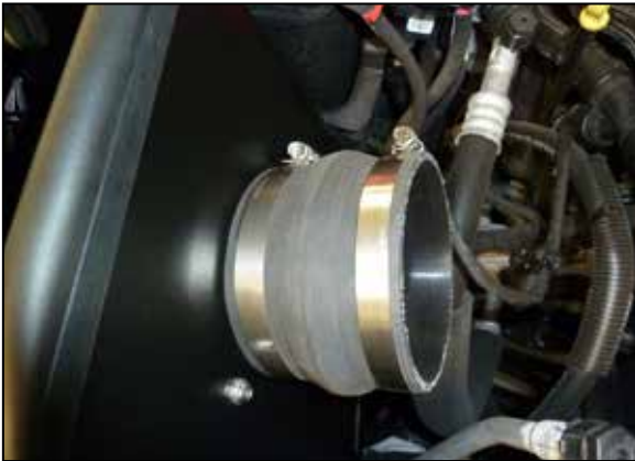
16. Install the provided hump coupler onto the filter adapter and secure with the provided hose clamp.
