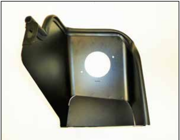
8. Install the provided edge trim onto the heat shield as shown. Some trimming of the edge trim will be necessary.
