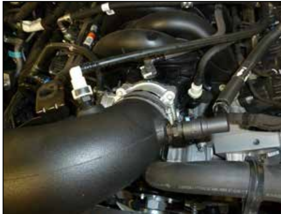
18. Reconnect the CCV hoses to the fittings installed into the K&N intake tube.
