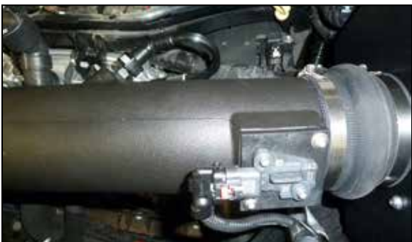
31. Reconnect the mass air sensor electrical connection.
