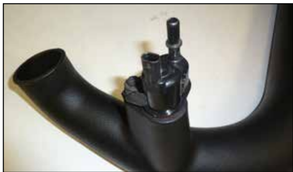
25. Remove the CCV solenoid from the factory intake tube and install it into the K&N intake tube using the factory bolt.
