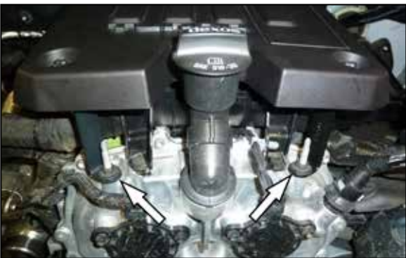
28. Install the engine cover onto the engine and secure the brackets to the factory mounting studs using the factory nuts.
