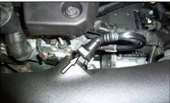
29. Connect the CCV tube to the quick connect fitting installed into the K&N intake tube.
