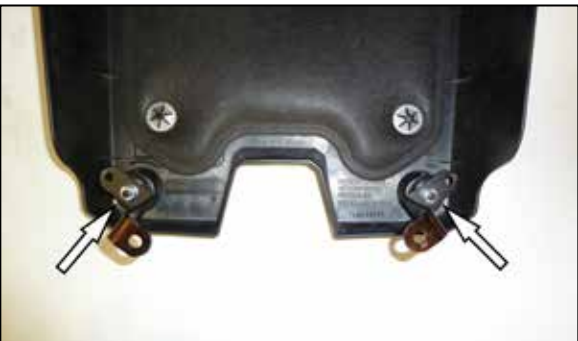
27. Using the factory bolts and the nuts provided, secure the two provided "Z" brackets to the engine cover as shown.
