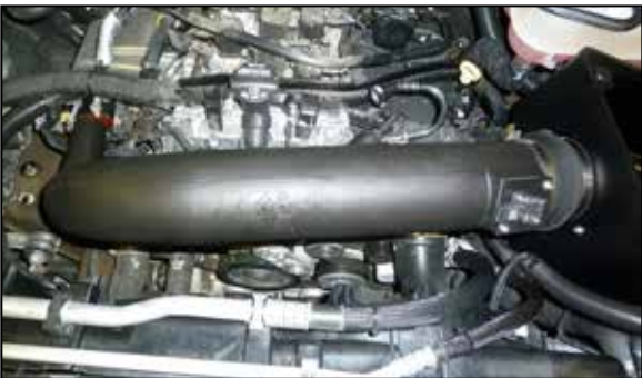
26. Install the intake tube assembly into the coupler at the air filter housing and then into the coupler at the turbo inlet, adjust the tube for best fit and then secure with the provided hose clamps.
