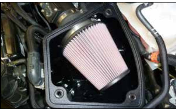
32. Install the K&N air filter onto the filter adapter and secure with the provided hose clamp.
