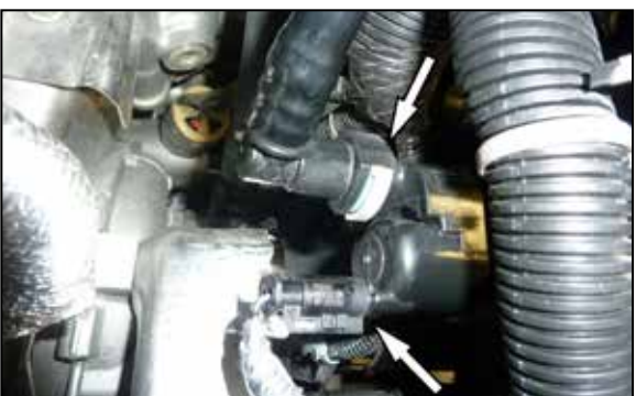
30. Connect the CCV tube to the solenoid and connect the electrical connection.
