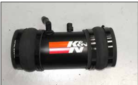
14. Install both coupling hoses (08418) onto the K&N intake tube as shown. NOTE: Install the hose as far onto the tube as possible to aid the installation onto the vehicle.
