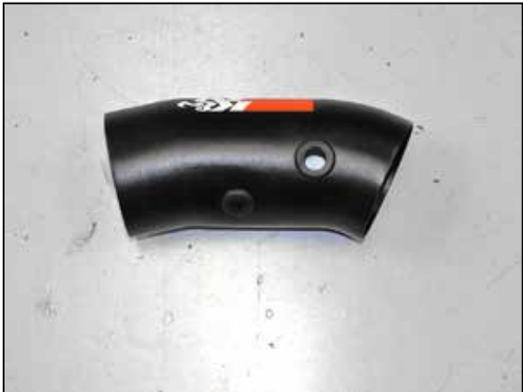
11. Install the two provided grommets into the K&N intake tube.
