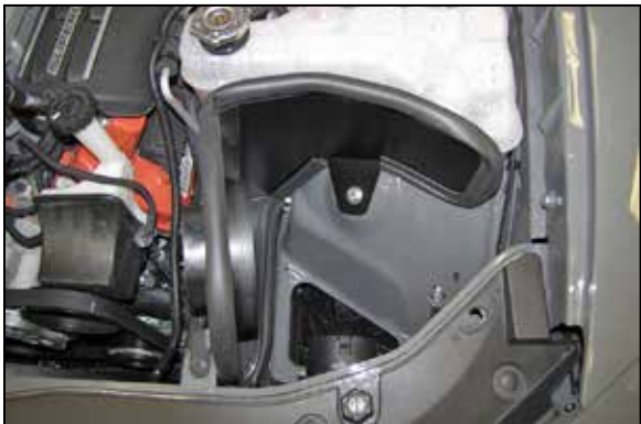
10. Install the heat shield assembly into the vehicle so the insert nut goes into the factory air box grommet mount. Secure the bracket to the core support with the factory bolt from step #6 and tighten the bolt into the insert nut.
