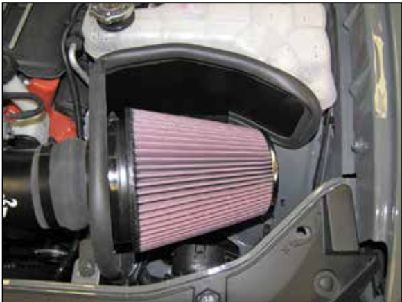
17. Install the K&N air filter and secure with the provided hose clamp. NOTE: DRYCHARGER #RF-1041DK is available separately and is recommended if the vehicle is to be used in inclement weather. Protection of the air filter is recommended while washing the vehicle as the filter is exposed under the hood grill.
