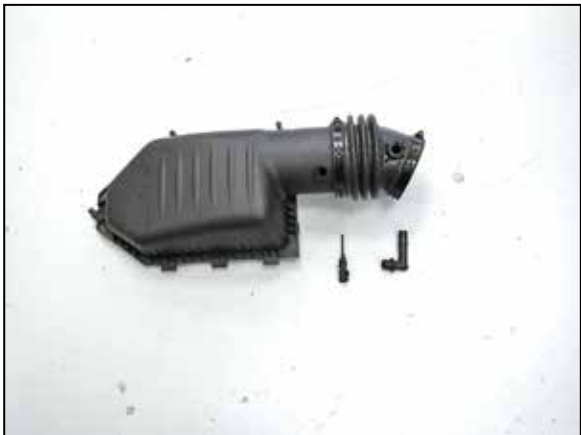
12. Remove the crank case vent and inlet air temperature sensor from the factory intake tube. NOTE: The inlet air temperature sensor is very fragile, use care while removing the sensor.
