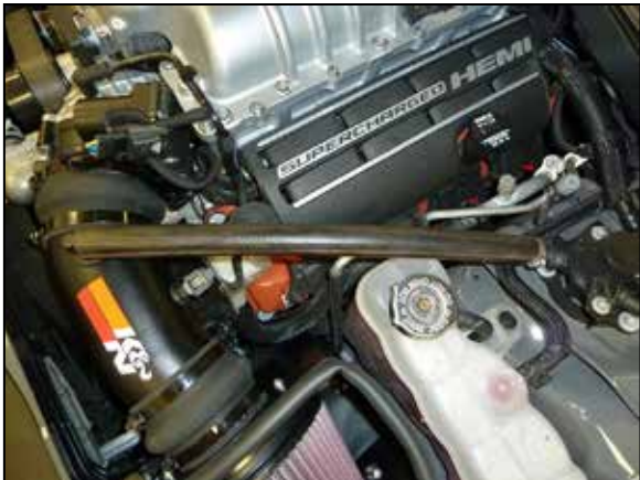
16a. On models equipped with the solenoid vent valve, install the provided crank case vent line and secure to the solenoid vent valve port using the provided hose clamp.
