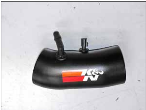
13. Install the crank case vent and inlet air temperature sensor into the K&N intake tube. NOTE: the inlet air temperature sensor is very fragile, use care while installing the sensor. NOTE: On vehicles with the crank case vent solenoid valve, install the provided 90° vent fitting in place of the factory fitting.
