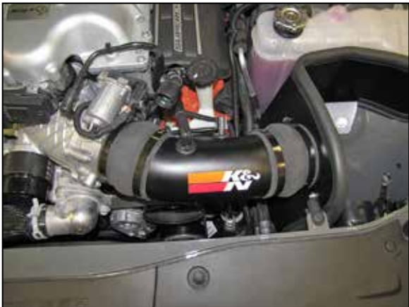
15. Install the K&N intake tube assembly into position, Slide the coupling hoses out and onto the throttle body and filter adapter. Then adjust the tube and hoses for proper fit and secure with the provided hose clamps.
