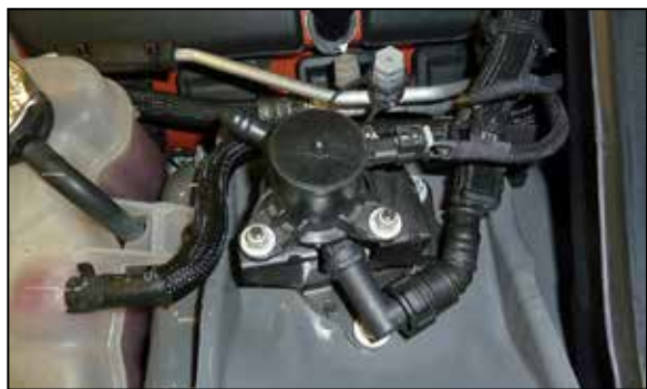
4c. Reinstall the solenoid valve onto the factory mounting bracket and secure with the factory hardware.
