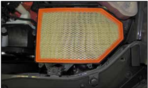
5. Remove the bolt securing the lower air filter housing to the core support and then remove the air filter housing from the vehicle. NOTE: It may be helpful to separate the fresh air duct from the air filter housing to aid its removal. The factory bolt will be reused in a later step. On Charger models, the fresh air duct will stay in the vehicle. NOTE: K&N Engineering, Inc., recommends that customers do not discard factory air intake.
