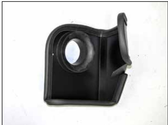
7. Install the provided edge trim onto the heat shield as shown. NOTE: Trimming of the edge trim will be necessary.
