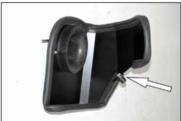
9. Install the Inserted nut onto the heat shield as shown.
