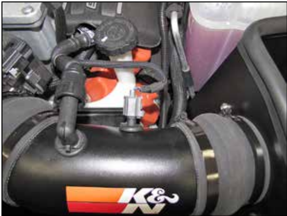
16. Reconnect the crank case vent hose and inlet air temperature sensor electrical connection.
