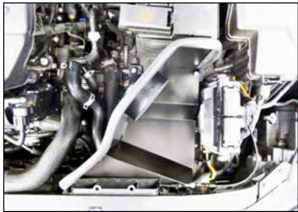
7. Install the heat shield into the vehicle and secure to the air filter housing mounting locations with the hardware provided.
