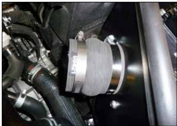
9. Install the hump coupler onto the filter adapter and secure with the provided hose clamp.
