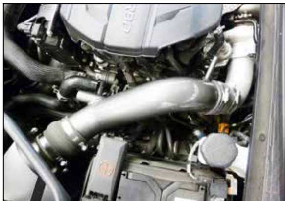
10. Install the K&N intake tube into the coupler, adjust for best fit and then secure with the provided hose clamp.
