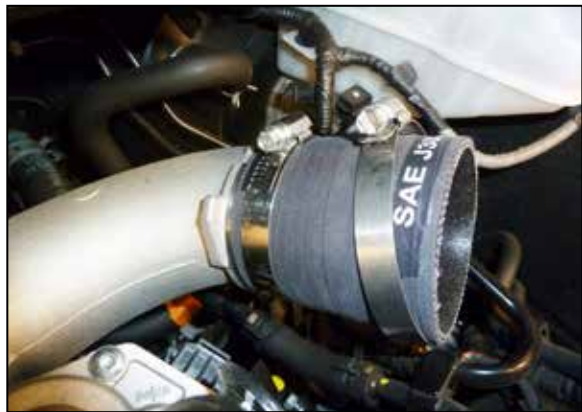
8. Install the step coupler onto the turbo inlet and secure with the provided hose clamp.
