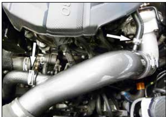
11. Connect the BOV hose and CCV hose to the K&N intake tube and secure with the factory spring clamps.
