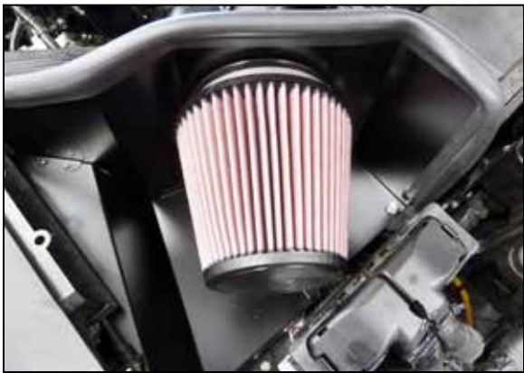
12. Install the K&N air filter onto the intake tube and secure with the provided hose clamp.
