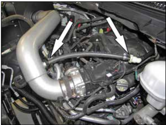
25. Install the crank case vent hose assembly onto the fitting installed into the K&N® intake tube and then connect the quick disconnect fitting into the factory connector as shown.
