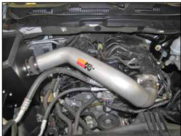
22. Install the K&N® intake tube assembly into the coupler hose at the filter adapter and then into the coupler hose at the throttle body. Adjust the tube for best fit and then secure with the provided hose clamps.
