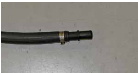
24. Install the provided quick disconnect fitting into the provided crank case vent hose and secure with the provided hose clamp.
