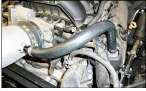
19. Install the provided CCV hoses onto the valve cover ports and connect the driver side hose to the K&N intake tube and secure with the provided hose
