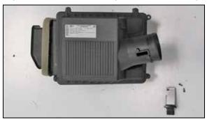
15. Remove the mass air sensor from the factory air box.
