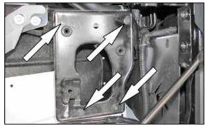
7. Remove the four bolts securing the air box mounting tray and then remove the tray from the vehicle.
