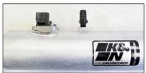
16. Install the mass air sensor into the K&N intake tube and secure with the provided hardware. Apply thread sealant to the CCV fitting and install it into the K&N intake tube.
