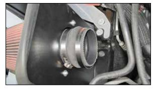
14. Install the coupling hose (08699) to the filter adapter and secure with the provided hose clamp.
