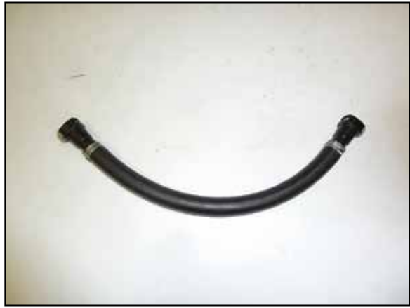
23. Install the provided quick connect fittings into the provided crank case vent hose and secure with the provided hose clamps.
