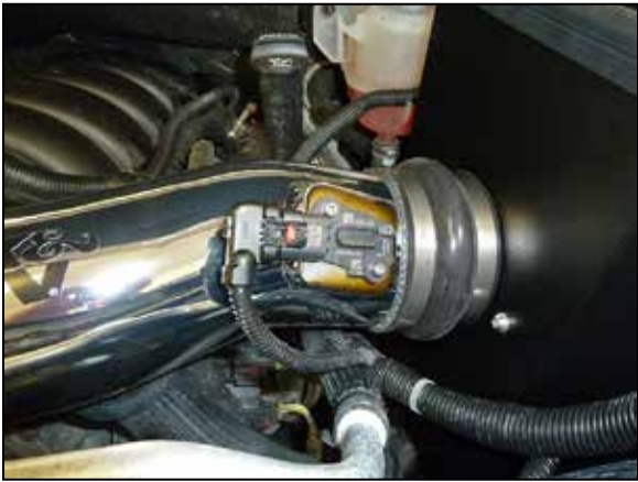
25. Connect the mass air sensor electrical connection.
