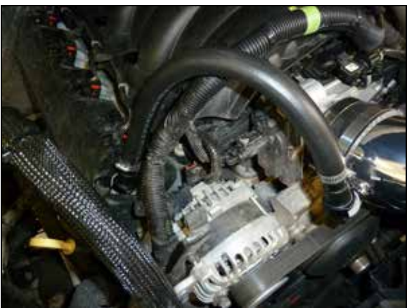
24. Connect the crank case vent hose assembly to the valve cover port and then to the fitting installed into the intake tube.
